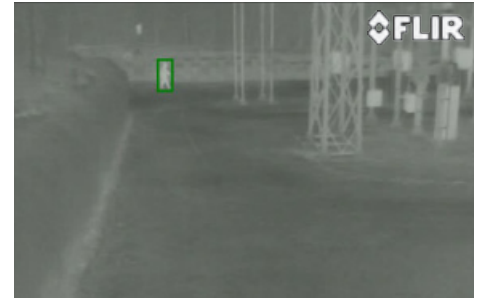
The FLIR SR-Series thermal imaging cameras installed at the Lyse Energy electrical substation can be used to detect man sized targets from hundreds of meters.
